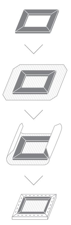
Migliorquadro canvas stretching machine is equipped to **stretch and staple** canvas on frame of different size from as small as **8"x8" up to 47"x47"**. To increasing productivity, the machine can **simultaneously finish multiple frames and canvas in the same size or width**.
